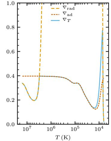
Figure 1: The dimensionless ( $\nabla_T$ ), radiative ( $\nabla_{\text{rad}}$ ) and adiabatic ( $\nabla_{\text{ad}}$ ) temperature gradients, plotted as a function of temperature  $T$  for a MESA model of the present-day Sun. The solar convection zone corresponds to the region where  $\nabla_{\text{rad}} > \nabla_{\text{ad}}$ .
