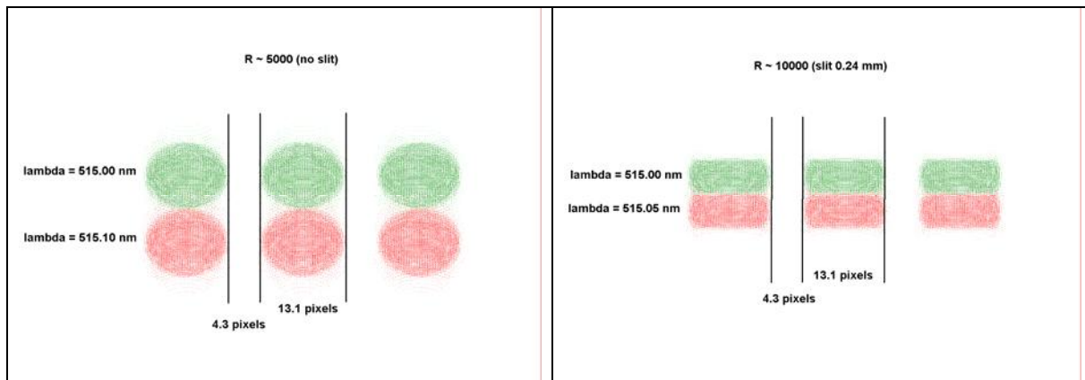
Figure 3: Simulation of spectral images in the centre of the detector to show spatial and spectral resolution for the final configuration. The separation between the spectra is 4.3 pixels, the spectra are 13.3 pixels wide. The left panel shows the separation of images for a spectral resolution of R \sim 5000 and no slit in the exit pupil of the microlens (diameter 500\mu\text{m} ); in the right panel the resolution is R \sim 10000 with a slit of 0.24\text{ mm} running over the exit pupils.
