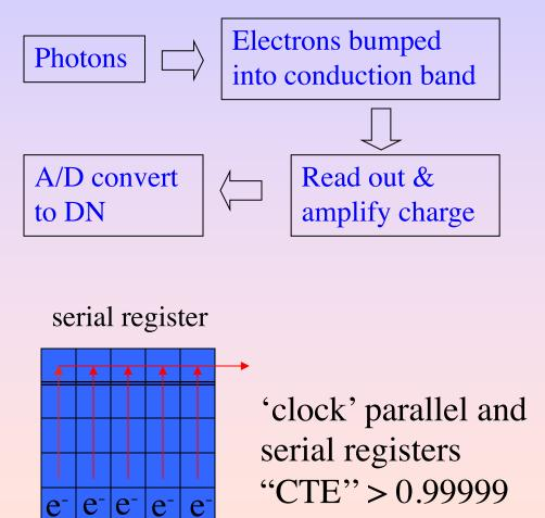
Silicon semiconductors with "gate" structure to produce little potential corrals or wells.
