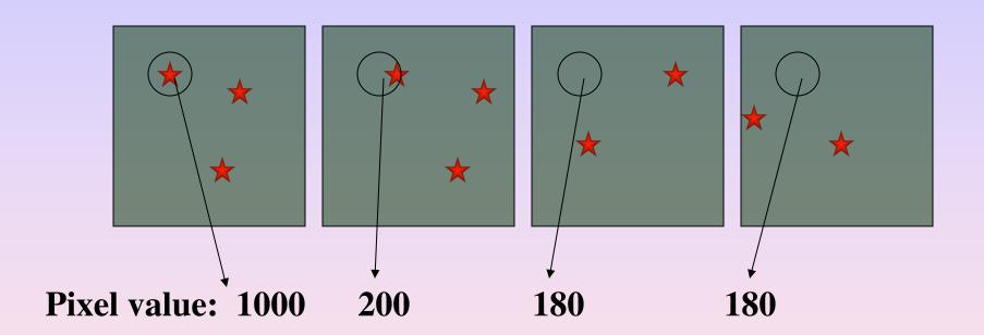
Average with minmax rejection, reject 2 highest value averaging lowest two will give the sky value. NOTE! Must normalize frames to common mean or mode before combining! Sometimes it is necessary to pre-clean the frames before combining.
